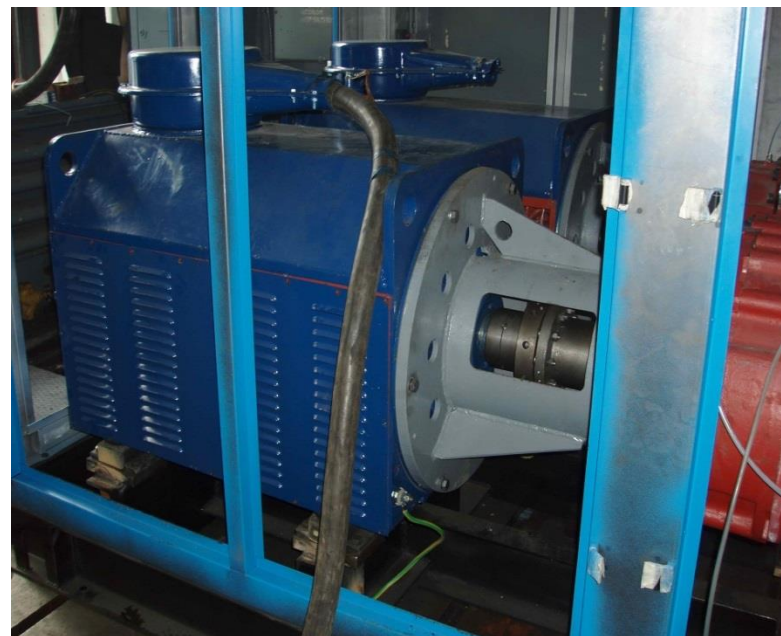
Motor of A5K-355-315-2Y3 type as a part of compressor
